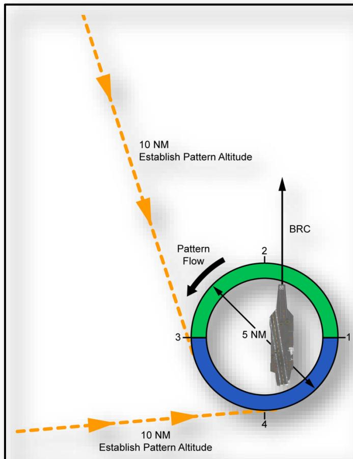
**Figure 2-3 Case I Port Holding Pattern Entry**
