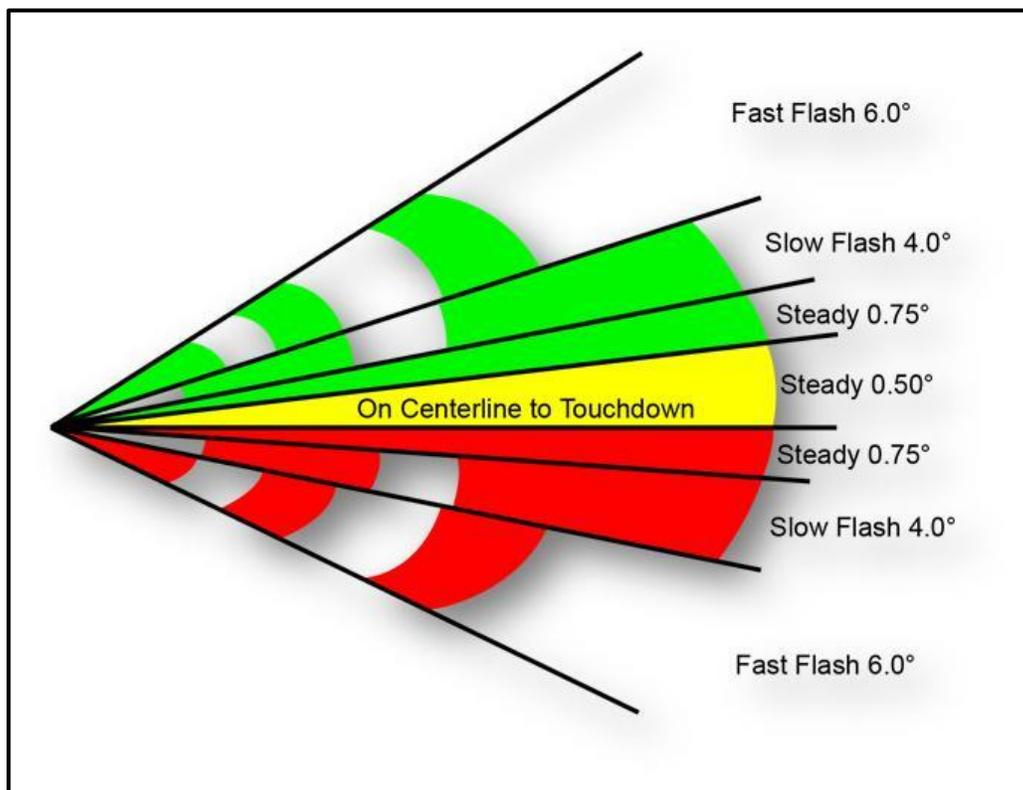
Figure 1-7 Long Range Laser Lineup System
