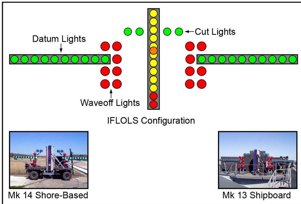
**Figure 1-4 Improved Fresnel Lens Optical Landing System (IFLOLS)**
