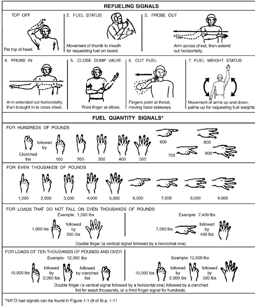
Figure B-11 Flight Deck Signals 11
