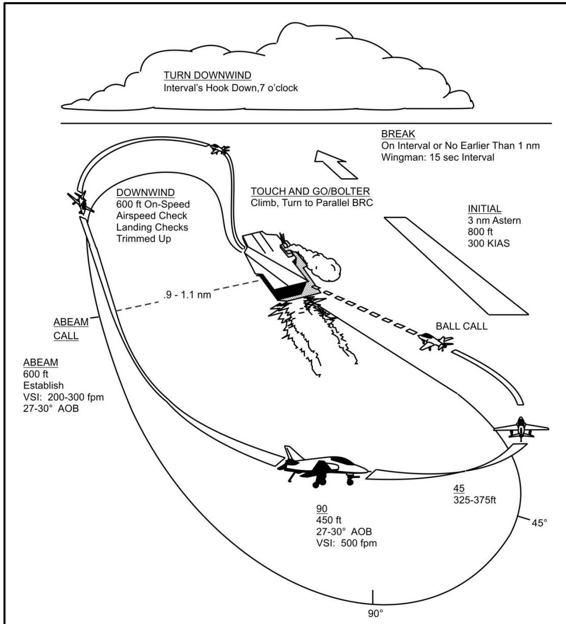
Figure 2-5 Carrier Landing Pattern
