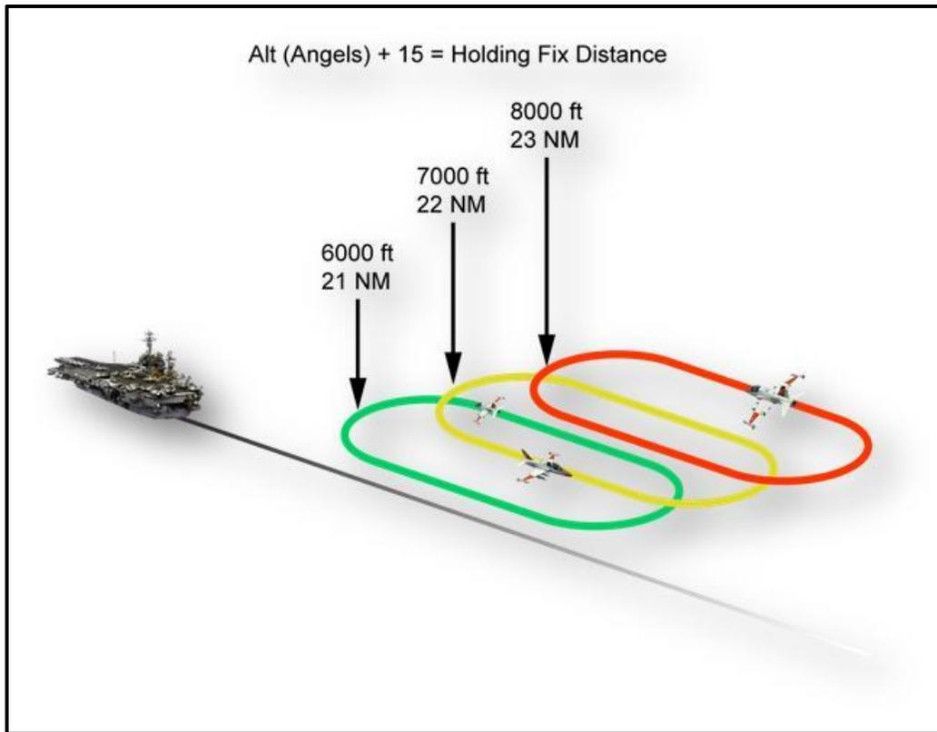
**Figure 2-6 Case II/III Marshal Holding**
