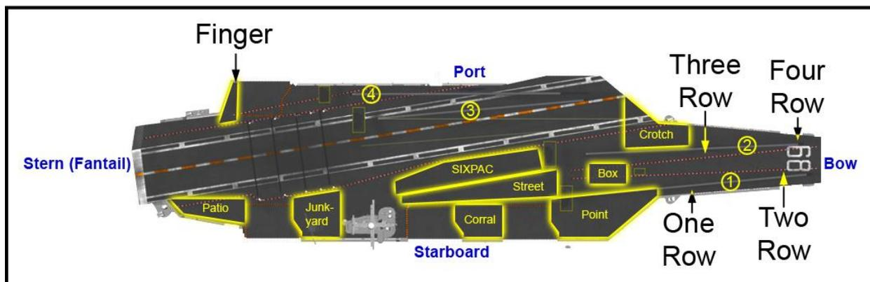
Figure 1-3 Flight Deck Layout
