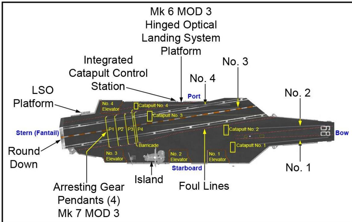
Figure 1-2 Basic Carrier Layout
